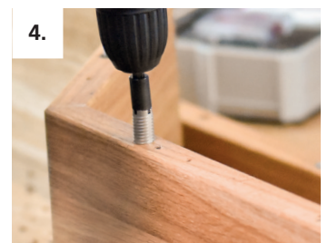
4. Screw the Invis Mx2 connector flush into the shelf
