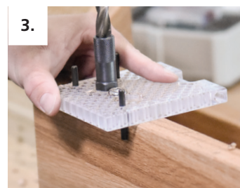
3. Add the drill holes to the shelf with the help of the drill jig
