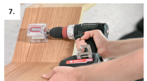
7. Join the components with the Minimag and a speed of 1200-1500 rpm min -1
