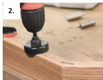
2. Fasten the stud with the insertion jig
