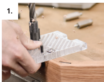
1. Drill precisely into the mounting strip thanks to the Rasto drill jig
